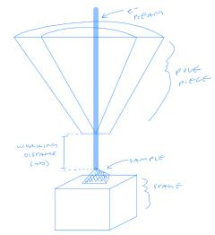
When the user is initially looking at the sample the microscope does not know that the working distance measured is from the bottom of the pole piece down to the sample. Therefore, going into the navigation page on the software and changing the z-axis direction from measuring the bottom up to measuring the bottom of the pole piece down will tell the microscope where the sample's surface is.
