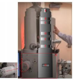
The main parts of the microscope are the column, chamber, a surface that holds the microscope, and then the user console. Within the column are the following:
